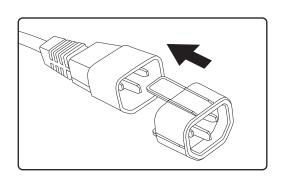
2. Connect the plug with the EZ-Lok Connector into the PDU by sliding it directly over and straight into the outlet.
