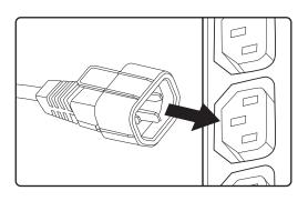
3. To disconnect the plug from the PDU, grip the plug and squeeze the EZ-Lok tab as you pull the cord from the outlet.
